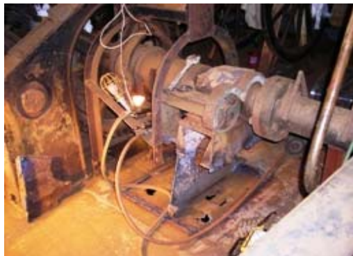
Steel Plate Below Steering Shaft Full Of Holes
